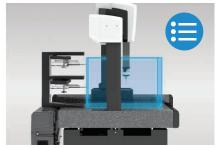
With the ProMax E option, ZEISS offers an automated probe changing magazine to guarantee the complete measuring volume during the changing process. It automatically moves into the measuring range and replaces the probe systems safely and accurately.
