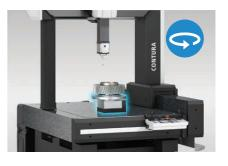
The new flexible rotary table can be installed in the measuring range as a surface-mounted variant when needed and can then be conveniently moved out of the measuring range again. This option enables measurements in four axes.
