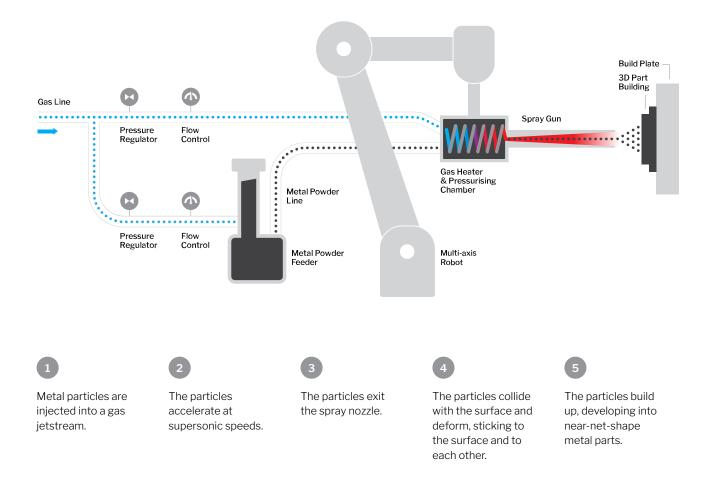
This process unlocks **limitless design possibilities** with minimal heat distortion. And because the materials keep their intrinsic properties, they're comparable or superior to cast and wrought materials.
