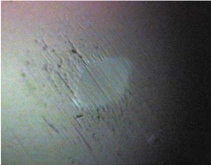
The scratches on the surface of this ruby ball are clearly visible
