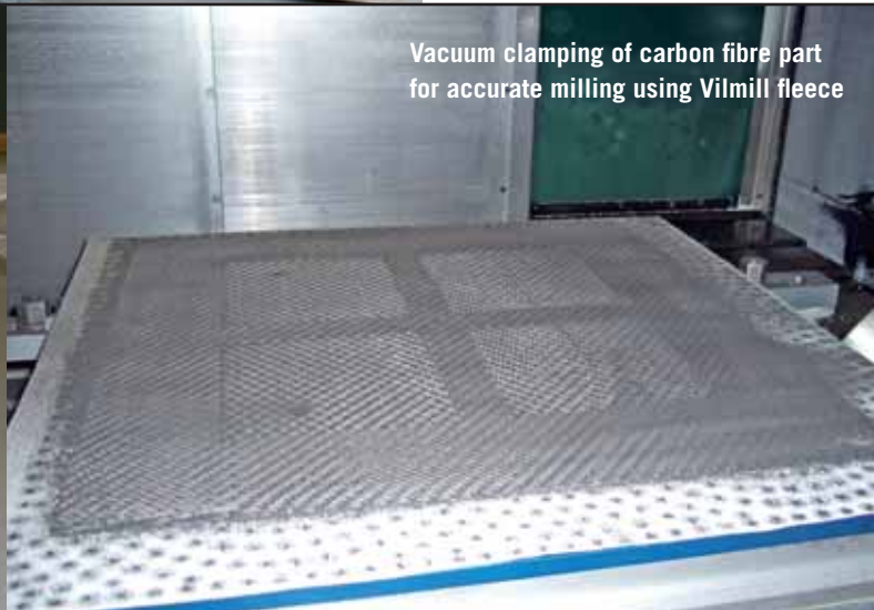
Grid hole type chuck with integrated Vilmill roller, surface area 1300x300mm
