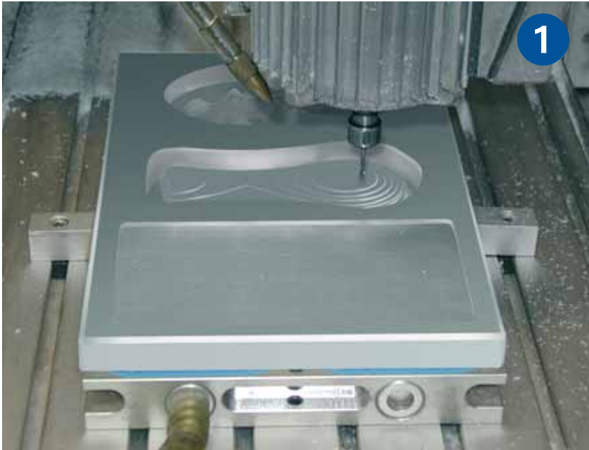
Left: First step is milling workpiece conventionally
