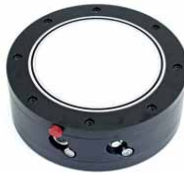
Independent vacuum chuck. Clamping of parts on chuck completely free of external supply lines. Battery, vacuum pump, controls, display and valves are all integrated
