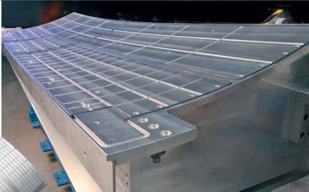
Vacuum fixture for clamping aircraft wing parts during friction-stir welding
