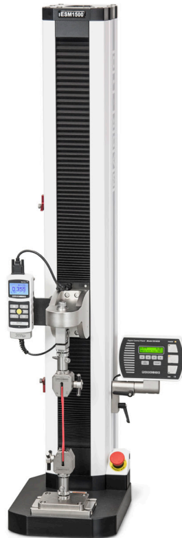
ESM1500 1,500 lbF [6.7 kN] 32 in [813 mm] travel
