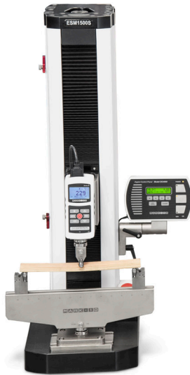
ESM1500S 1,500 lbF [6.7 kN] 14.2 in [360 mm] travel
