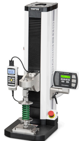
ESM750S 750 lbF [3.4 kN] 14.2 in [360 mm] travel
