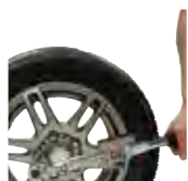
Completion of tightening process with Blue signal.
