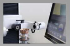
Measure grinding wheel packs with the ZOLLER **»smile«** measuring machine
