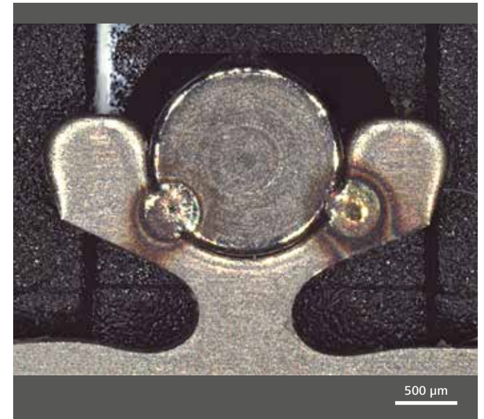
Laser welds Objective: 1.6×, expanded depth of field, LED ring illumination
