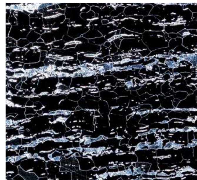
Steel structure, darkfield, objective: EC-EPIPLAN 20x/0.4
