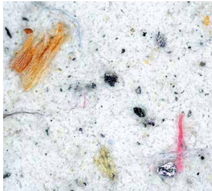
Metallic, non-metallic particles and fibers on filter membrane microscope: ZEISS Axio Imager.Z2m Objective: EC Epiplan-NEOFLUAR 10x/0.25 Camera: ZEISS AxioCam MRC
