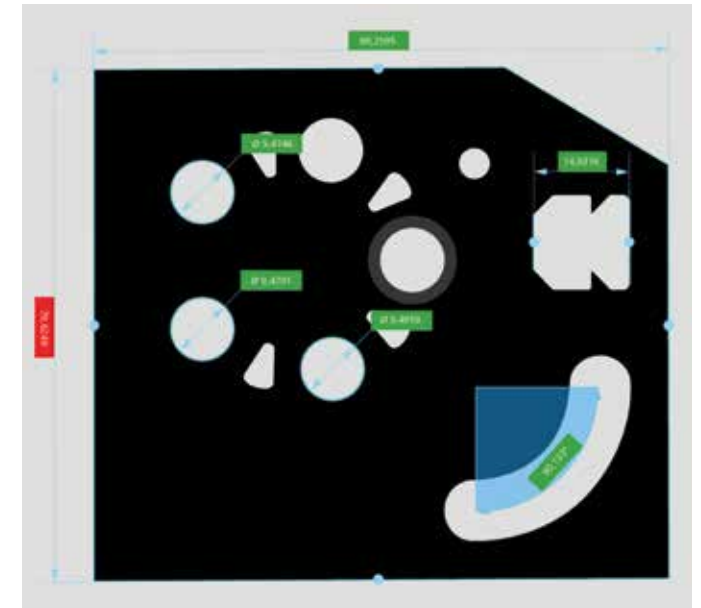
Results are superimposed directly at the dimensioning arrows on the image. Color coding immediately indicates that values are within tolerance.
