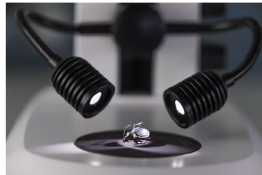
For sample preparations in reflected light, the double spot illumination with self-carrying goosenecks is optimal. It creates half-shadow effects that lead to a good 3D impression without overly dark shadows. During dissections the specimen stays illuminated even if the manipulating hand covers one of the spots.
