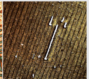
Laser-crystallized silicon on glass, EC Epiplan NEOFLUAR 5x/0.13
