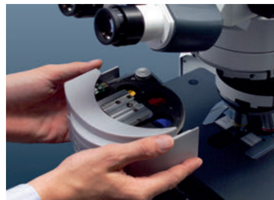
Simply fast: the change from manual to motorized reflector turret
