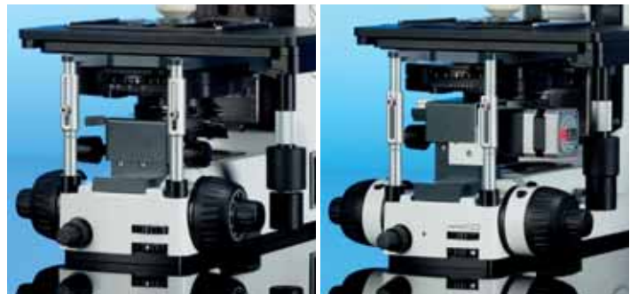
The control elements for focus drive, stage drive and condenser drive, for the selection of visible or infrared light, for adjusting the light field diaphragm, the regulation of light intensity and for all contrast techniques in transmitted-light are positioned at the very front of the stand. On the motorized stand (right) all the motors can be controlled with the keyrings.
