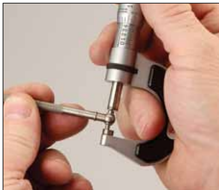
After establishing hole size with a telescoping gage, actual size is determined by measuring over the contacts with an outside micrometer.
