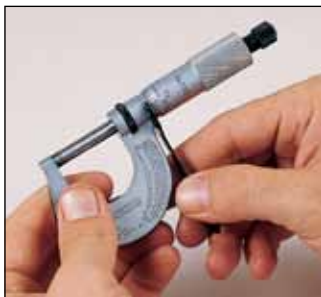
Illustrated: Adjusting for zero reading.
