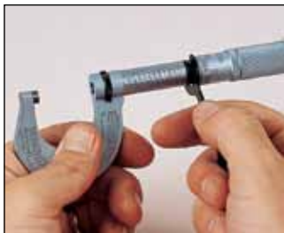
Illustrated: Adjusting spindle play.
