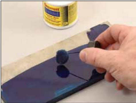
Blue layout dye being applied by brush.
