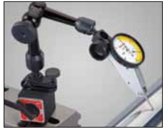
709B Dial Test Indicator attached to a 660 Magnetic Base Indicator Holder in an application to check for roundness.
