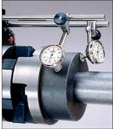
For a quick check of runout, lathe operator uses universal dial test indicator mounted in tool post.
