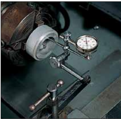
Checking lathework with dial test indicator. Tool post holder holds indicator securely in position.
