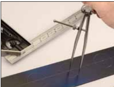
For precise layout of three identical circles, this mechanic uses 6" spring dividers.
