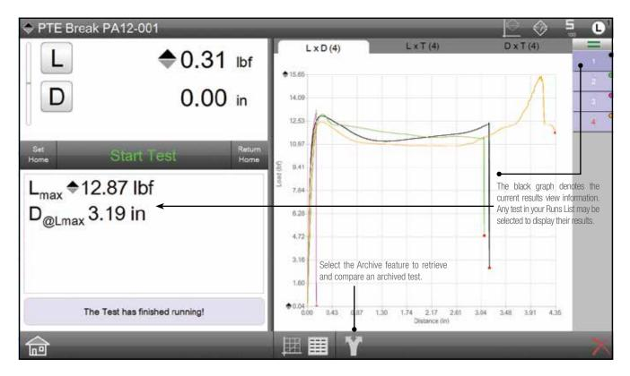
Compare the graphical results of multiple tests that you select. Individual graphs are color-codes and referenced to the test in the Runs List. You can also retrieve archived tests for making a graphical comparison. For example, you can compare a "benchmark" result from a year ago to a current result.
