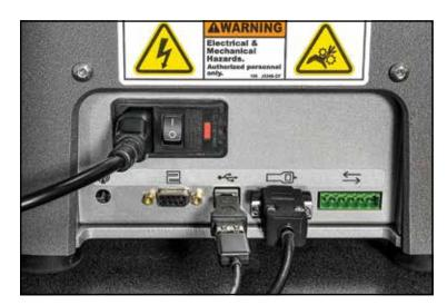
Interface connections and communications are clearly shown on the back panel. Source power may be 100-240V- no jumpers required or configuration needed.
