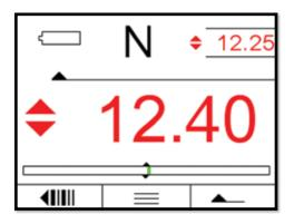
**Tolerance View** When a tolerance is used, out-of-tolerance results display in red.
