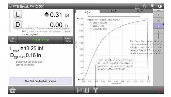
When the test concludes, your L1 software shows your results in numerical and graphical formats. Essential measurements are displayed an easy-to-interpret formats. You can Start and Stop a test using the touchscreen display; manually set the home position and return the crosshead to home position, an zero your load (L) and distance (D) measurements.
