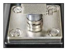
The standard base plate features four hole patterns for mounting fixtures; M4, M6, M10 and M12. An optional imperial base plate features #10-32, 5/16-18, 1/4-28, and 1/2-20. The base plate can be easily positioned to ensure correct sample alignment.
