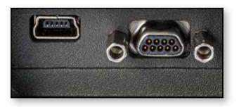
The USB connection is used for charging the battery or for transmitting data to a personal computer. The RS-232 cable is used for connection to the FMM Digital Tester. The DFC also has Bluetooth<sup>®</sup>.
