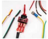
The "make and break" load for an Insertion/extraction testing is performed electrical switch can be measured and the peak load is measured when the switch closes/opens. This type of application can be tested on keypads, membranes and other materials that utilize a resistance change.
