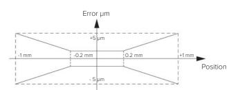
Example: ±1 mm transducer with 0.5% reading error
