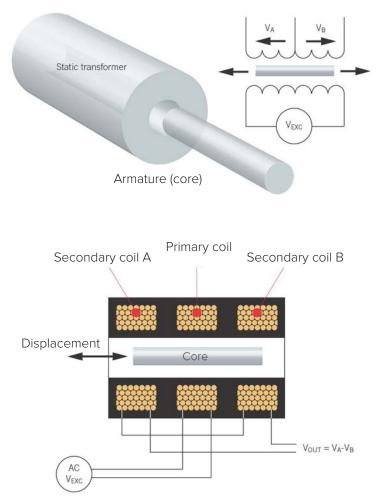
The output of an LVDT is a linear function of the displacement over its calibrated range. Beyond this range the output becomes increasingly non linear. Measurement range is defined as  $\pm$  distance from the transducer zero or null position.
