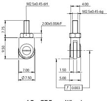
1.5 x Ø7.5 mm Wheel Tip Material Part no. Steel 008305-027
