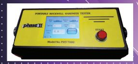
Load Cell, Closed Loop, Rockwell Hardness Tester!
