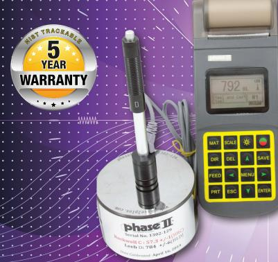
The PHT-3500 can perform tests that easily convert to the most popular hardness scales, including Rockwell, Brinell, Vickers, Shore, etc.
