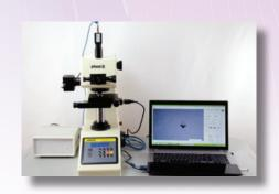
Motorized X-Y Stage w/Controller and Measurement Software
