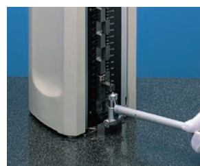
Using height master to set bore gage
