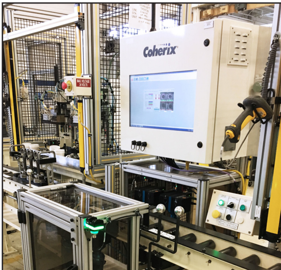
Robust3D™ Piston Assembly error-proofing inline installation
