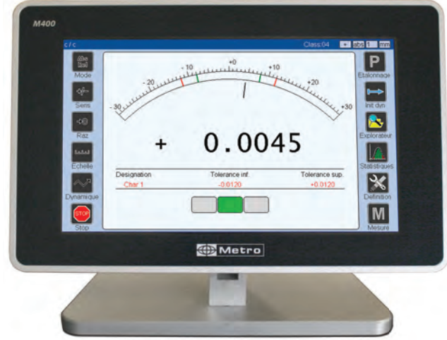
Simple gauging display mode with the needle indicator
