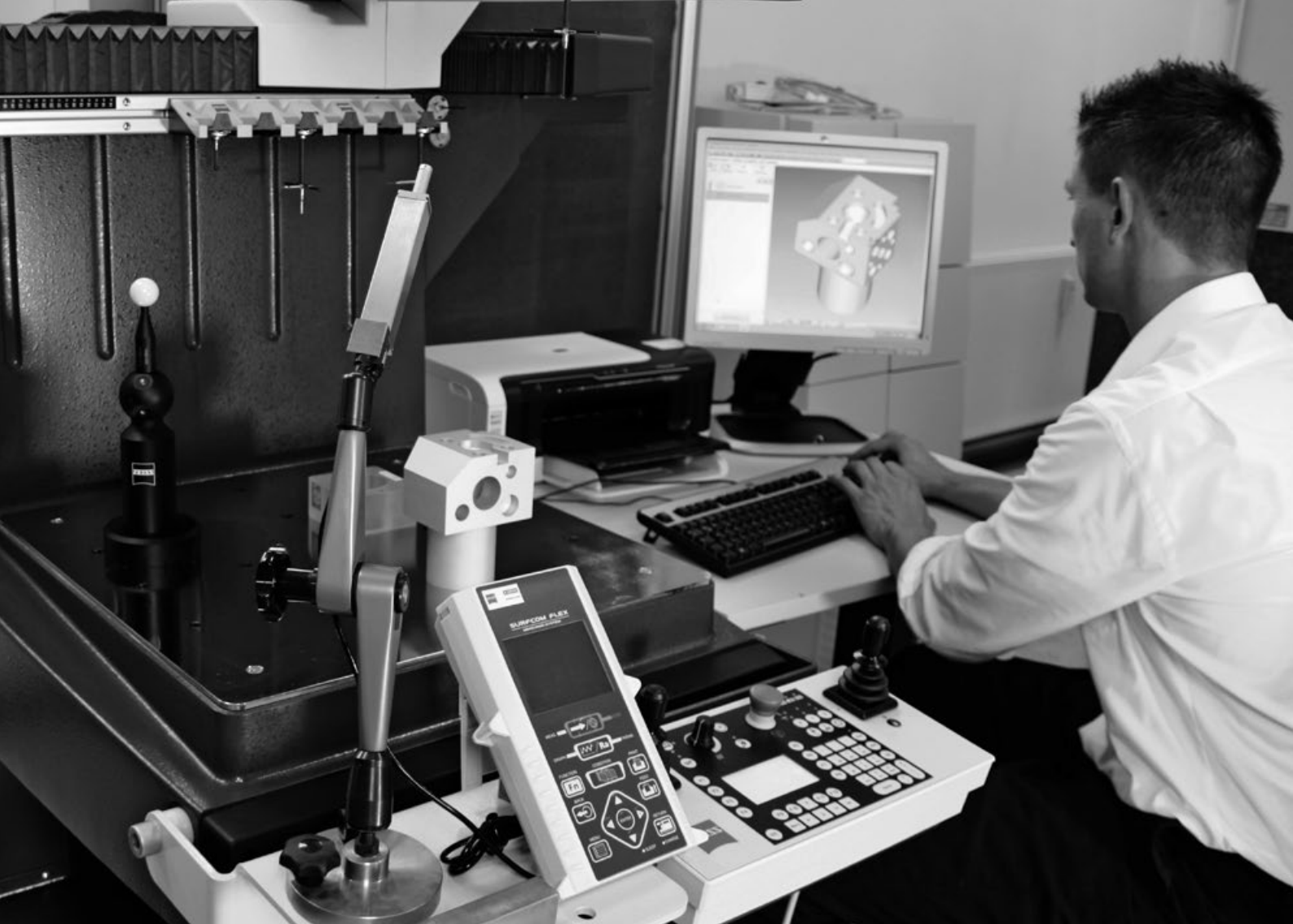
Form, size, position and roughness inspection in one run and one report.
