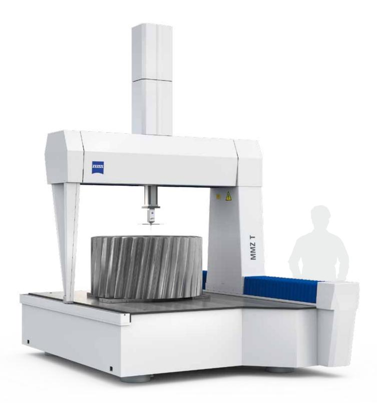
With a measuring range of up to 14.8 m<sup>3</sup>, the MMZ T line is the largest of the table bridge-type measuring machines from Carl Zeiss. It allows the highly precise measurement of large gears directly on the shop floor. The open design enables easy loading with a crane. A crane interlock to protect against collisions is a standard feature.
