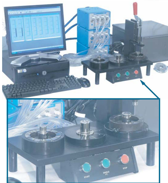
Three Spindle Inspection station checks bore size, O.D. size, I.D. to O.D. concentricity, and bore to face perpendicularity on machined bearing housing. Uses 3 quad AEK air/electric converters coupled to CWK-2 computer. (Images Above)
