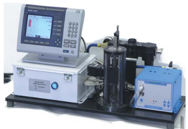
Canister Bore Inspection Station. Stepper motor driven slide moves an air probe to measure internal diameter at multiple locations. Integrated with WGC's AEK & GageChek. (Image at right)
