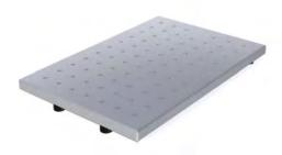
This 300 x 200 grid pallet with changer system has a 25 mm M6 hole line spacing. As a result, user-defined workpiece holding fixtures with bracket clamping systems or other elements can be assembled. You will find suitable clamping material in our clamping kit.
