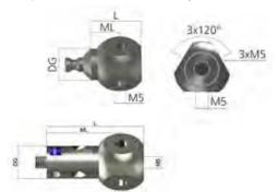
The cube comes with four M5 threads, three of which are arranged at an angle of 120°. The star piece is inserted in a cone receiver. As a result, you can quickly assemble adjustable stylus systems.
