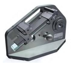
The Multisensor-Check is a procedure for the standardized checking of coordinate measuring machines (CMMs) with tactile/optical sensors. The universal calibration artifact is supplied with the associated control and analysis software. The Multisensor-Check can be used to check coordinate measuring machines in accordance with DIN EN ISO 10360-2 and VDI/VDE 2617 Sheet 6.1:
