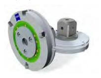
These adapter plates for VAST® come with an ID-chip for reliable identification by the ZEISS CMM. Furthermore, they are equipped with a 20 mm cube that has already been aligned. Five M5 connections can accommodate styli and extensions. The reference adapter plate is marked with a red ring.
