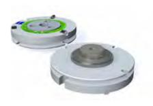
These adapter plates for VAST® come with an ID-chip for reliable identification by the ZEISS CMM. In addition to this, they are equipped with an M5 holder. An M5 stylus or an extension with a diameter of 20 mm can be attached to this in a vertical direction. As a result of their flat design, they are ideal for use with the Z measuring range.
